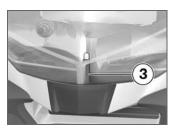
• Remove bulb socket **3** from the headlight housing from be-
